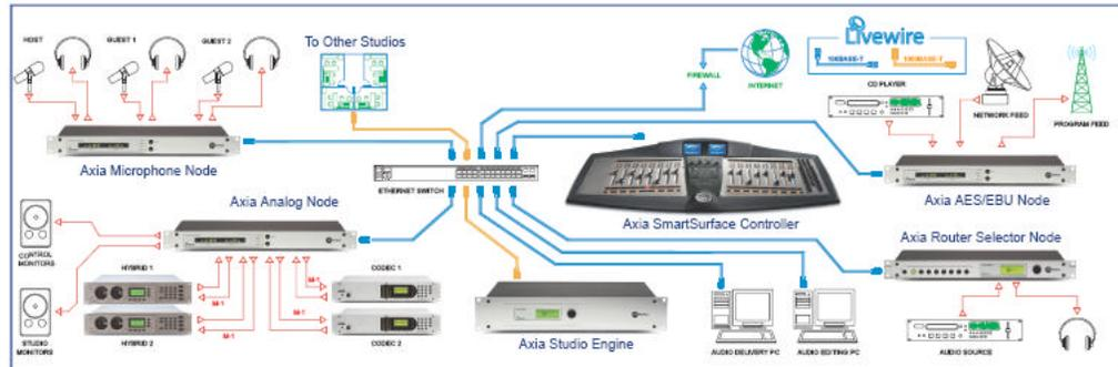
Typical connection scheme for an IP-Audio network
